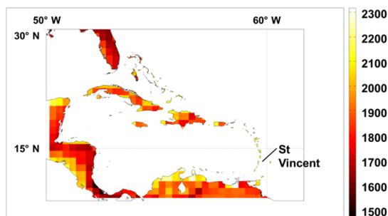
**Figure 1: Solar Map Caribbean Area,** Global horizontal radiation in kWh/m<sup>2</sup>\*year, shows the excellent solar power potential, especially on the eastern Caribbean Islands such as St Vincent [1].
