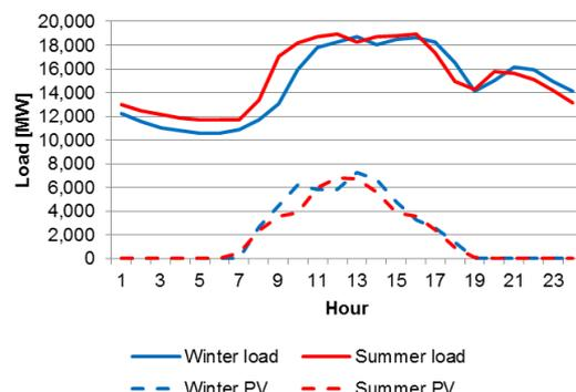
**Figure 2: Load and PV power generation profile for St Vincent in 2010,** The load profiles for an average summer and winter day in the year 2010 are shown, in addition the potential PV production by 10 MW installed PV for the same days. The shape of the curves reveals the advantage of the daily PV power generation without seasonal differences [7], [8].
