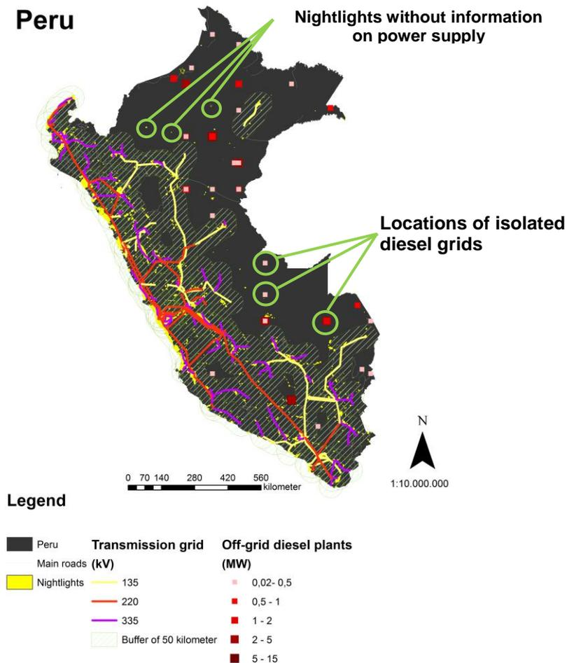
Figure 1: Peru - Diesel mini-grids, nightlights and national transmission grid
