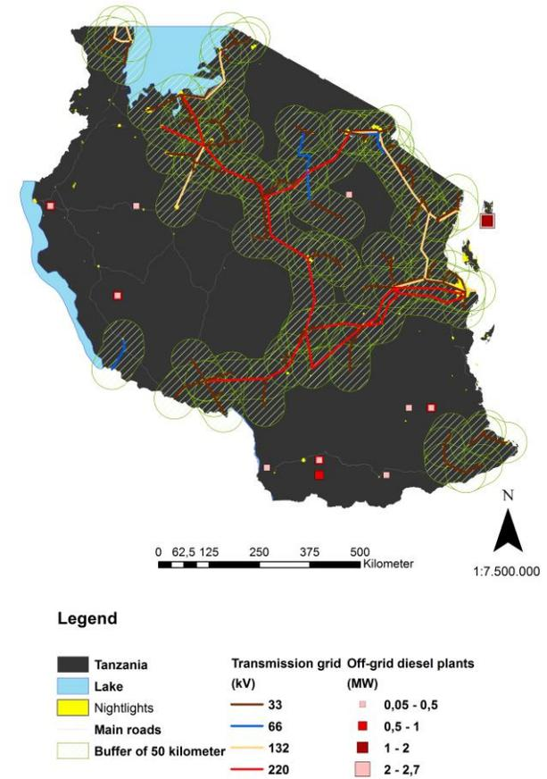
Figure 3: Tanzania - Diesel mini-grids, nightlights and national transmission grid
