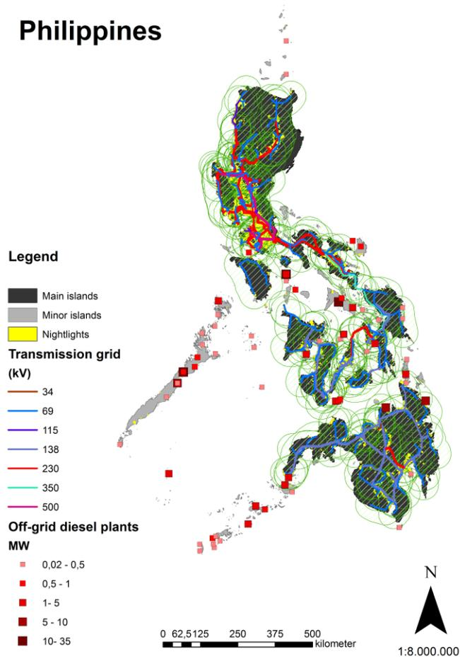
Figure 2: Philippines - Diesel mini-grids, nightlights and national transmission grid
