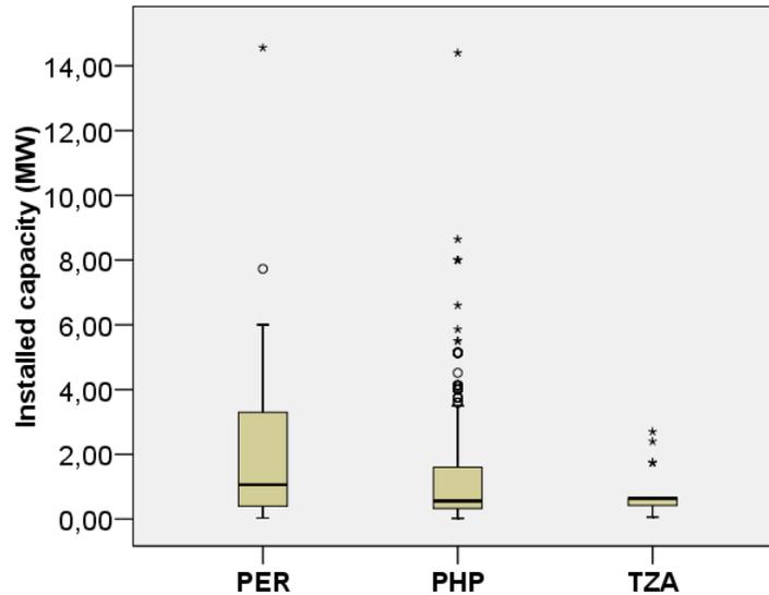
**Figure 5: Boxplot showing the distribution of off-grid diesel generator sizes in Peru, the Philippines and Tanzania**
