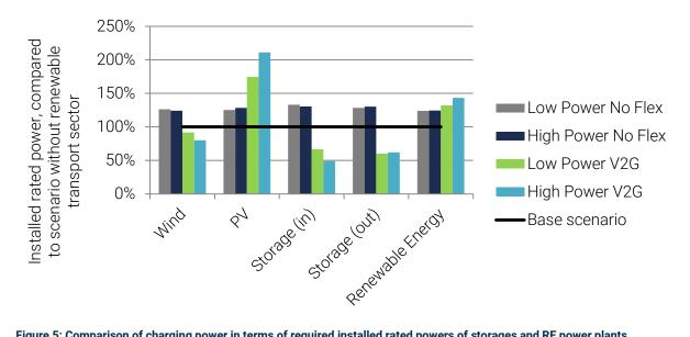
Figure 5: Comparison of charging power in terms of required installed rated powers of storages and RE power plants
