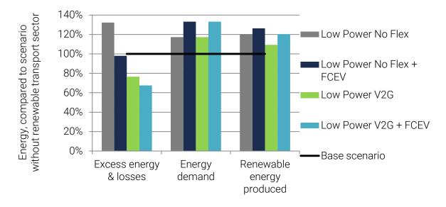
Figure 7: Comparison of different FCEV scenarios in terms of required energy production, excess and losses as well as demand
