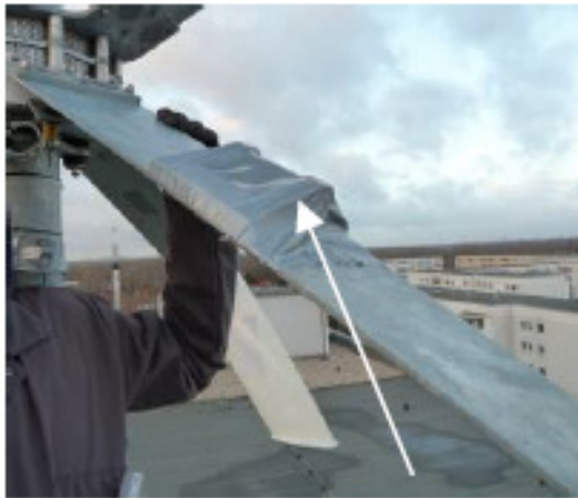
Figure 7: Test masses temporarily fixed at the blade holders for 2-plane balancing measurement at older SWT version
