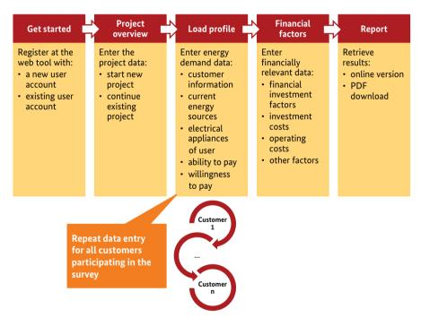
Figure 12: Graphical illustration of mini-grid builder and data required
