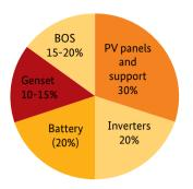
A typical cost structure of PV-diesel-battery hybrid mini-grid systems is shown in Figure 10. Some tools include default values as cost suggestions, which can be adapted (i.e. the mini-grid builder, see Chapter 3.2) and others only consider the users' input.
