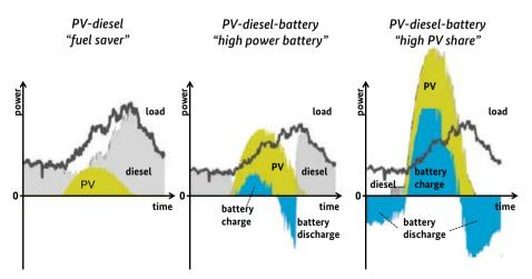
Figure 9: Illustration of different operation modes of hybrid systems, adapted from [Fricke 2015]
