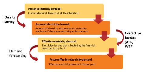
Figure 5: Steps in order to assess the (future) effective electricity demand needed for system sizing
