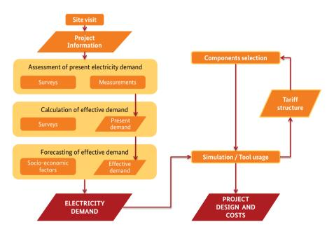
Figure 3: Flow chart of the sizing process
