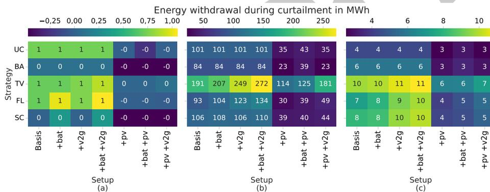
Fig. 4 Effect of strategy and setup on the customers energy withdrawal during curtailment in MWh within each grid area N1-N3 from left to right.
