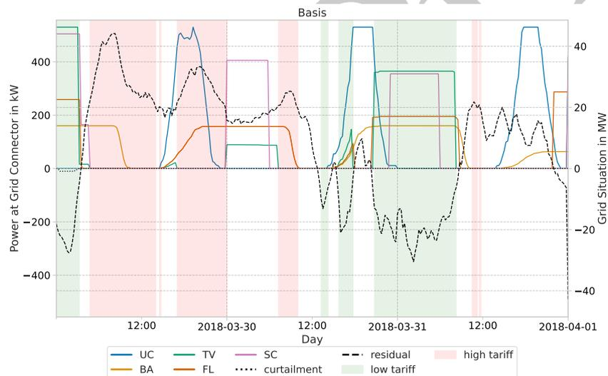
Fig. 3. Load profiles of the charging strategies (left axis) in grid area N3 with balanced grid situation (right axis).
