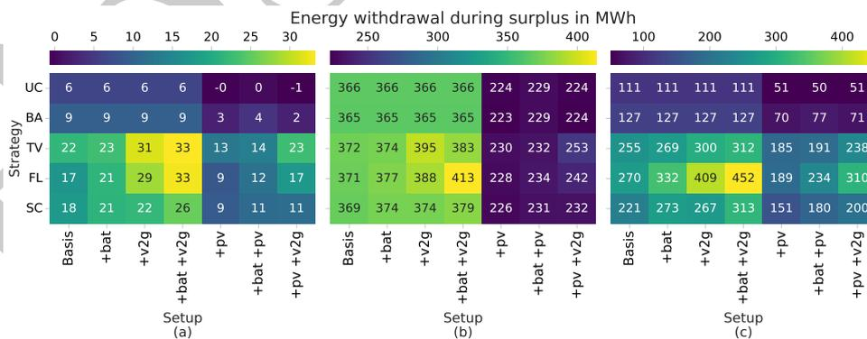
Fig. 5 Effect of strategy and setup on the customers energy withdrawal during generation surplus in MWh within each grid area N1-N3 from left to right.
