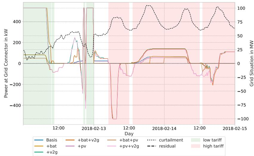
Fig. 10 Residual peak load of grid area N1 on 13.02. at 18:00 overlaps with local consumption, when TV uses V2G feature.
