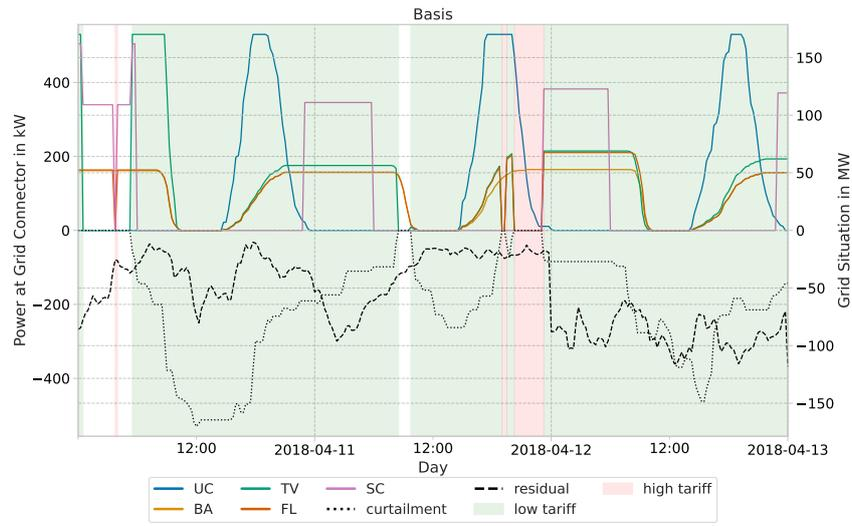
Fig. 2 Load profiles of charging strategies (left axis) in grid area N2 with high generation surplus and curtailment (right axis) resulting in (green) low tariff windows.
