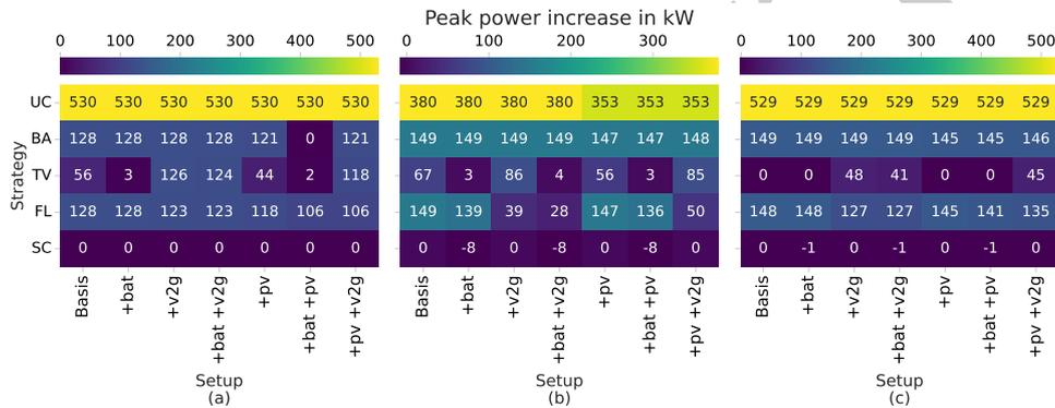
Fig. 6 Effect of charging strategy and setup on peak power increase in kW within each grid area N1-N3 from left to right, respectively.
