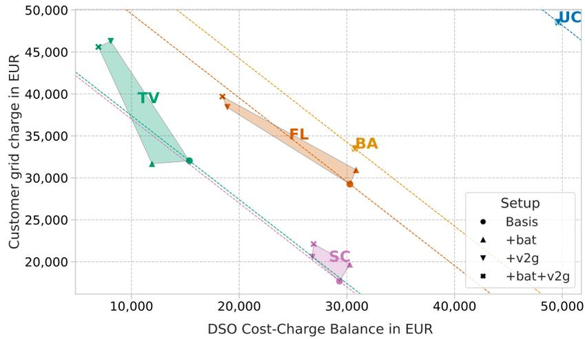
Fig. 7 Comparison of grid charge paid by the customer and the resulting balance of grid cost components and grid charges for the DSO as calculated in (1) and (3) for grid area N1: The values are highlighted by strategy (colour + guiding hull) and setups (marker type), the dotted reference lines visualises the influence of a changing grid charge on the DSO balance given otherwise constant costs components for each *basis* setup.
