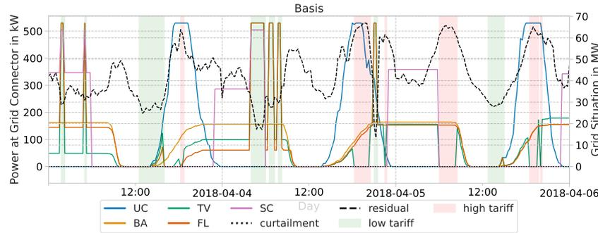
Fig. 1 Load profiles of charging strategies (left axis) in a three-day example of grid area N1 (right axis) showing high residual load and no curtailment.
