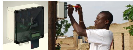
Figure 4: Load Management and Accounting Unit (LAU) [17].
