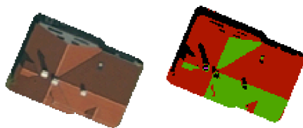
Figure 2: Original orthophoto clipped by the building footprint (left) and classified output after supervised image classification [black=shadow, red=non suitable, green=suitable, pink=obstruction] (right)
